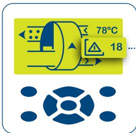
Space for the alphanumeric indicator for displaying unit faults.
